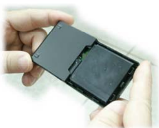
Step 2 Open the cover of battery
